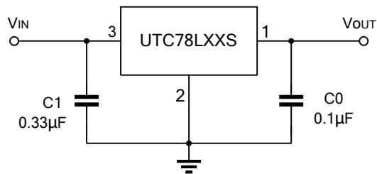
Notes: 1. To specify an output voltage, substitute voltage value for "XX".
