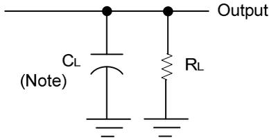
Note:  $C_L$  includes probe and jig capacitance.
