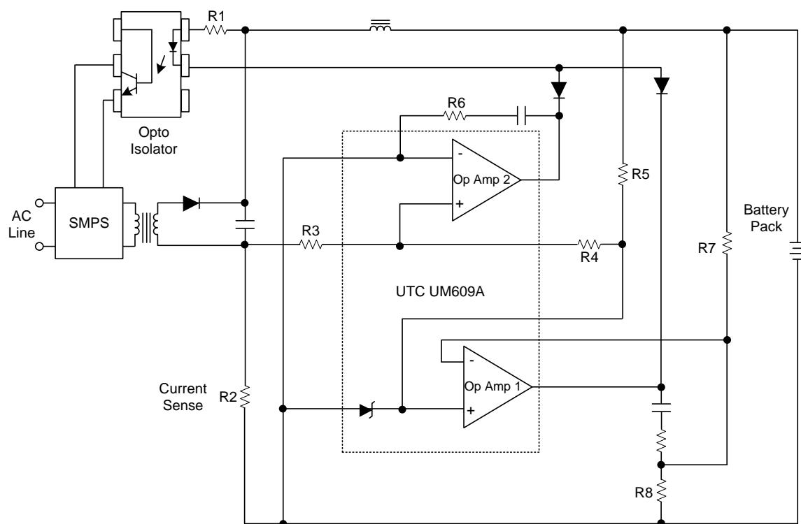
$$V_{OUT} = V_{REF} \times \frac{R_7 + R_8}{R_8}$$
