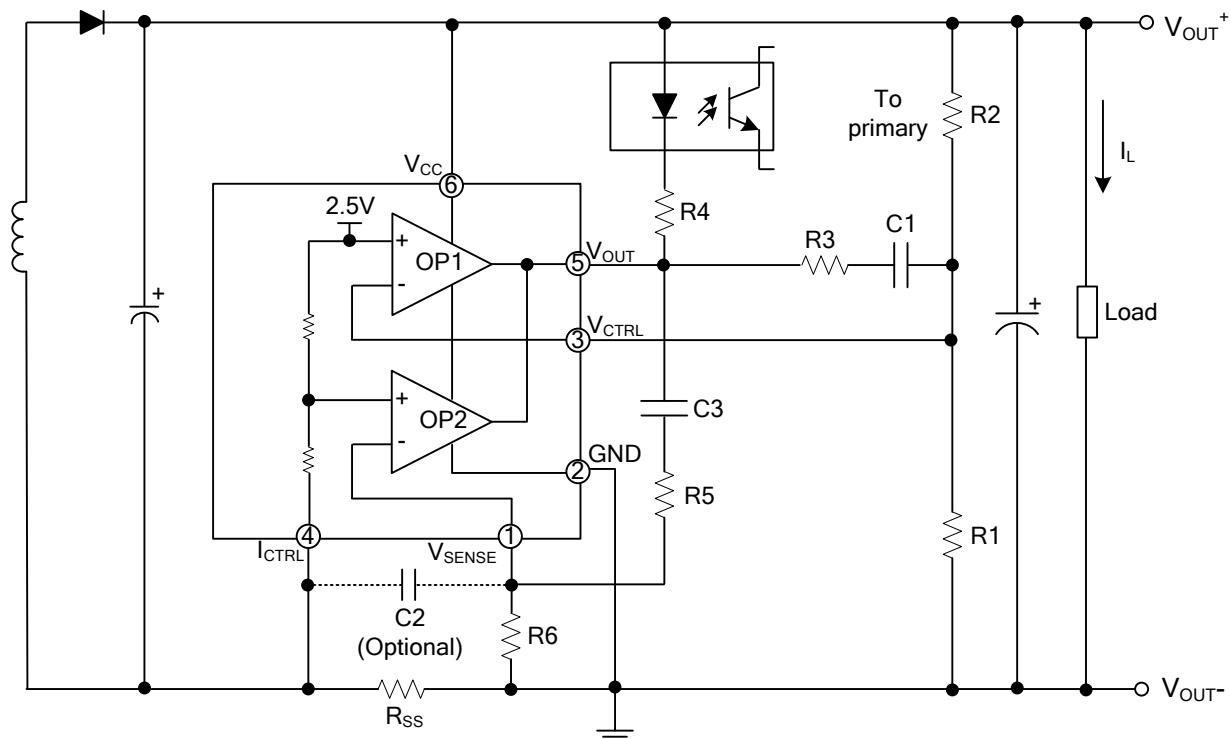
$$V_{OUT} = V_{REF} \times \frac{R_1 + R_2}{R_1}$$
