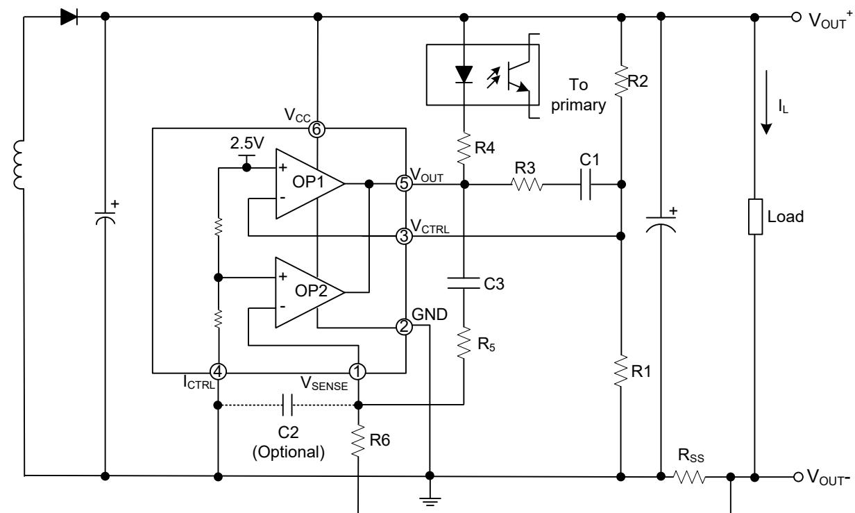
$$V_{OUT} = V_{REF} \times \frac{R1 + R2}{R1} - (I_L \times R_{SS})$$
